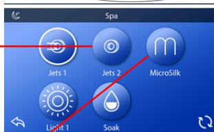
**MicroSilk®:** If equipped with this option, touching the MicroSilk button will turn on this special feature and run for 30 minutes. You will know it's on when a white ring is present around the button. Note that all other pumps will shut off after a few minutes in order for the feature to work as designed. Touching the button again will turn off the feature and allow control of the other pumps to be resumed.
