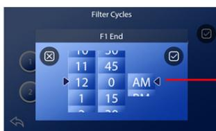
4. Use your finger to slide the scale up or down to the desired hours, minutes and AM/PM. Once selected, press the “check” mark to lock
