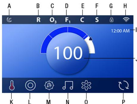
NOTE: References B through I are system indicators only. References A and, K through P, are functioning indicators that are activated when touched.
